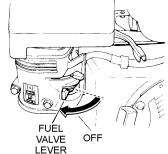
Figure 16. Fuel Valve Lever (OFF)
